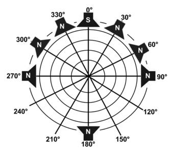
Figure 1. The test setup for the OLSA measurement during the directional microphone evaluation. Speakers labelled with S indicate the direction from which the speech material was coming from. Speakers labelled with N indicate from where noise was coming from.
